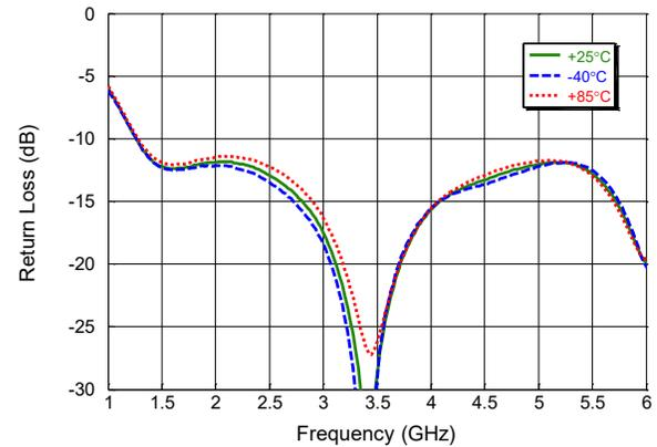
**RF<sub>OUT</sub> Port Return Loss over swept Frequency (& Temp.) in High Gain Mode**
