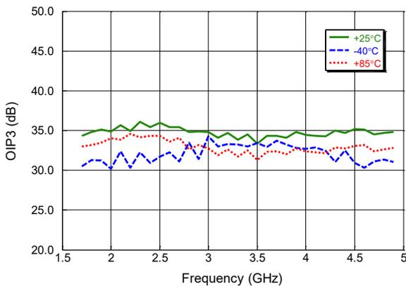
**OIP3 over swept Frequency (& Temp.) with  $P_{OUT}$ /Tone = 3 dBm & 11 MHz tone spacing in LGM.**
