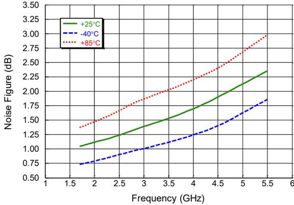
**LNA Noise Figure over swept Frequency (& Temp.) in Low Gain Mode**
