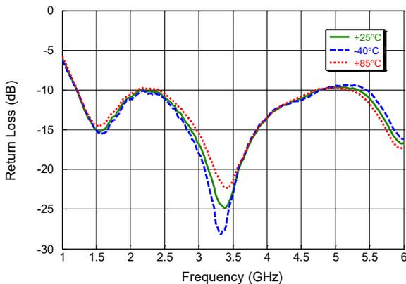
**RF<sub>IN</sub> Port Return Loss over swept Frequency (& Temp.) in Low Gain Mode**
