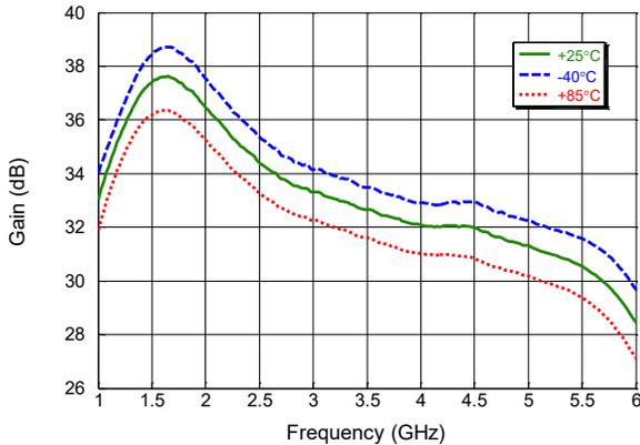
**LNA Gain over swept Frequency (& Temp.) in Low Gain Mode**
