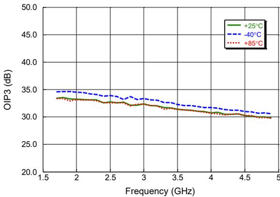
**OIP3 over swept Frequency (& Temp.) with  $P_{IN}$ /Tone = -25 dBm & 10 MHz tone spacing in LGM.**
