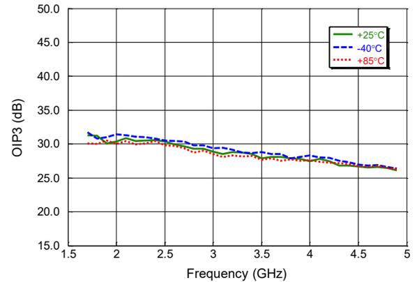
**OIP3 over swept Frequency (& Temp.) with  $P_{OUT}$ /Tone = 10 dBm & 11 MHz tone spacing in HGM.**
