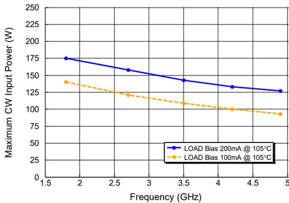
**ANT to LOAD Input Power Derating Curve over Frequency @ 120°C Case Temp**
