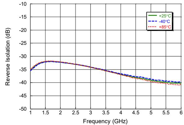
**RF<sub>IN</sub> to LNA<sub>1IN</sub> Isolation over swept Frequency (& Temp.)**
