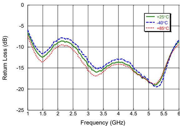
**RF<sub>OUT</sub> Port Return Loss over swept Frequency (& Temp.) in Low Gain Mode**
