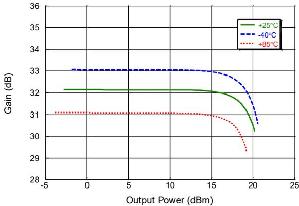
**LNA Gain over swept Output Power (& Temp.) at 3.5 GHz in Low Gain Mode**
