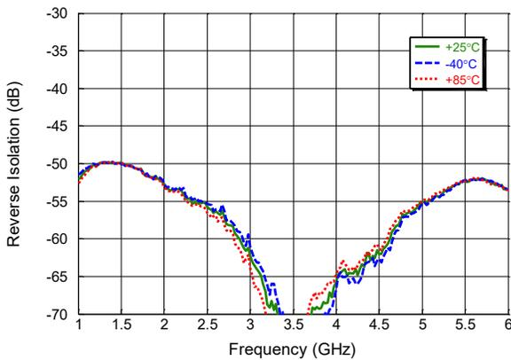
**LNA<sub>1IN</sub> to RF<sub>OUT</sub> Isolation over swept Frequency (& Temp.) in Low Gain Mode**
