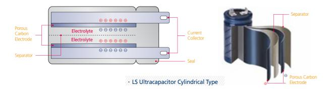
LS Materials provides optimal package design to provide the best in performance and reliability.
