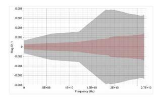
S11\_mag measured on a  $50\Omega$  termination SP-35-MM-36-LP shown in red; leading global competitor shown in grey
