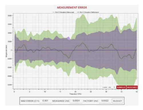
Figure 2. Normalized amplitude response between user-characterized and factory-characterized standard including uncertainty boundaries.
