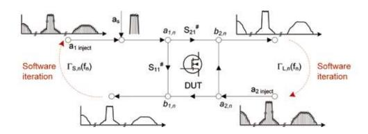
Figure 7 Software iteration of  $a_1$  and  $a_2$  to converge on desired impedances
