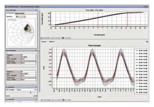
Output Current Waveforms at Constant Input Power Under Varying Load Impedances
