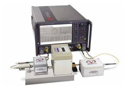
Typical setup for performing high-speed noise parameter measurements.
