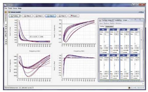
Linear Model Comparing Measured And Optimized Data
