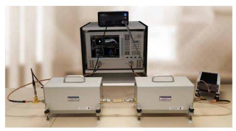
Pulsed DC and RF Load Pull bench architecture
