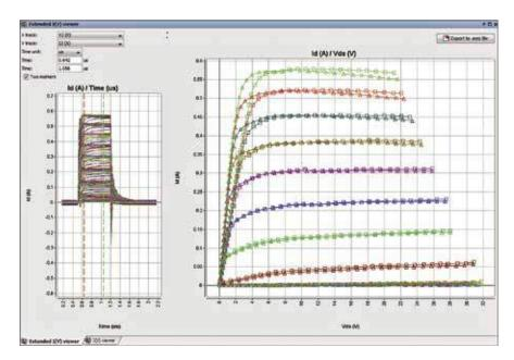
Pulsed IV Curves Plotted at Different Times with Pulse
