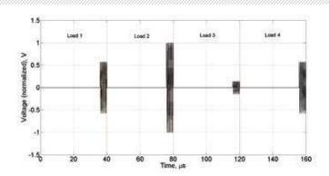
Figure 10 stitched modulated  $a_2$  signal representing multiple single-tone pulsed-CW reflection coefficients waveforms
