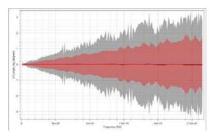
S11\_phase measured on a short circuit termination SV-35-FM-38 shown in red; leading global competitor shown in grey
