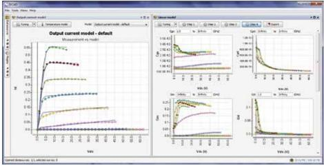
Multi-Bias Capacitances and Transconductance Model Extraction
