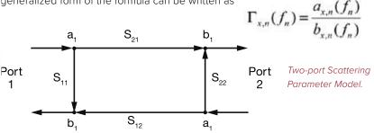
A closer examination of the formula  $\Gamma_L=a_2/b_2$  reveals that there is no limitation on separating the sources of  $a_2$  and  $b_2$ . It is obvious that  $b_2$  is the wave coming from the device, of which we have no direct control; however  $a_2$  need not be a reflected version of  $b_2$  but can be a new signal entirely!
