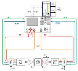
Figure 6: Simplified schematic of a load-pull architecture controllable with MMW-STUDIO LP
