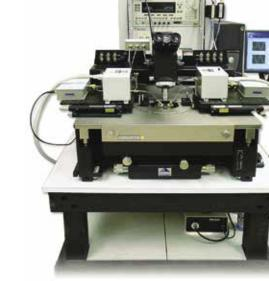
MT900N Series Fully Integrated 2.4mm 50 GHz LSNA Measurement System.
