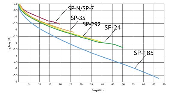
Maury StabilityPlus™ 36" Cable Assembly Typical Insertion Loss
