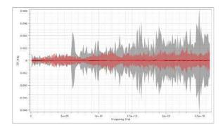
S11\_mag measured on a short circuit termination SV-35-FM-38 shown in red; leading global competitor shown in grey
