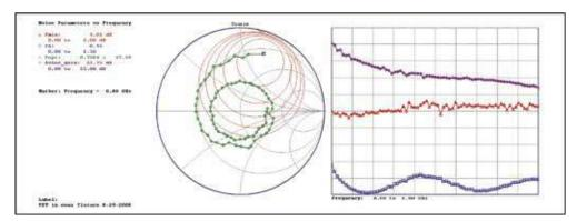
Measured noise parameter data using MT993B01 (no smoothing).
