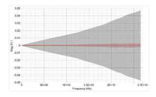
S11\_mag measured on a short circuit termination SB-SMA-MM-36 shown in red; leading global competitor shown in grey
