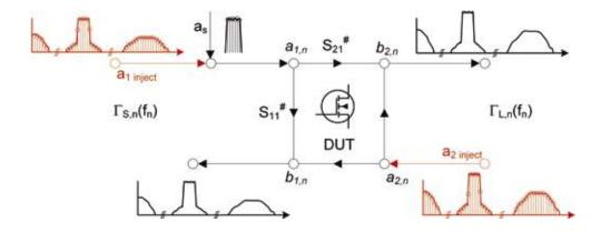
Figure 6 Active tuning a, and a, signals
