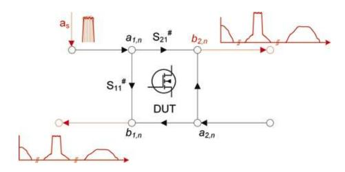
Figure 5 Injected as signal and resulting b, and b, waves
