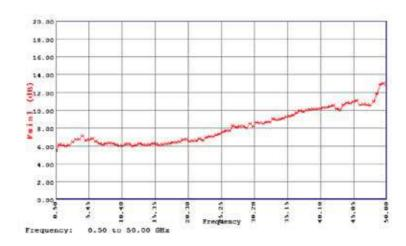
Figure 4. Typical Noise Receiver Calibration Using MT7553B03
