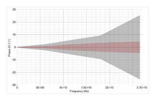
S11\_phase measured on a short circuit termination SB-SMA-MM-36 shown in red; leading global competitor shown in grey
