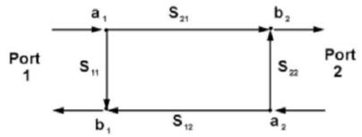
Figure 4: Two-port representation of a DUT
