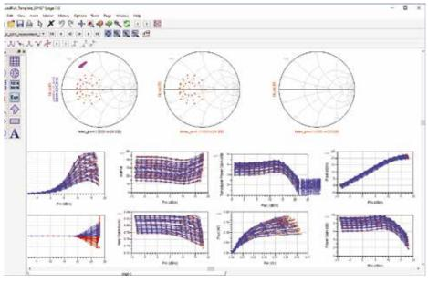
ADS Comparison of Measured and Modeled Performance Parameters
