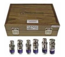
Maury precision BNC VNA calibration kits include each of the calibration standards and tools shown in the tables at the right. Between-series adapters are sold separately.
